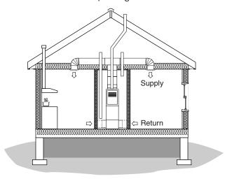
Balance the air pressure in the house and provide spot ventilation for non-vented combustion appliances, such as gas stoves.
