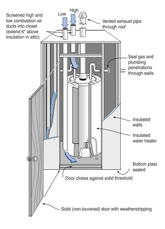
A closed combustion closet is, "a little piece of the outside located in the middle of the home". Fresh air for combustion is provided from sources not connected with the living space.
