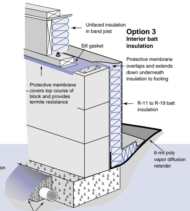
Perforated drainage pipe is embedded in gravel, covered with filter fabric, and located at lower perimeter of foundation footing to provide drainage.
