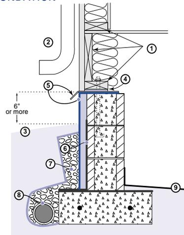
5. Install a protective membrane, such as an EPDM-type membrane, to serve as a capillary break that reduces wicking of water from the masonry wall. This membrane, in addition to metal flashing, can serve as a termite shield.
