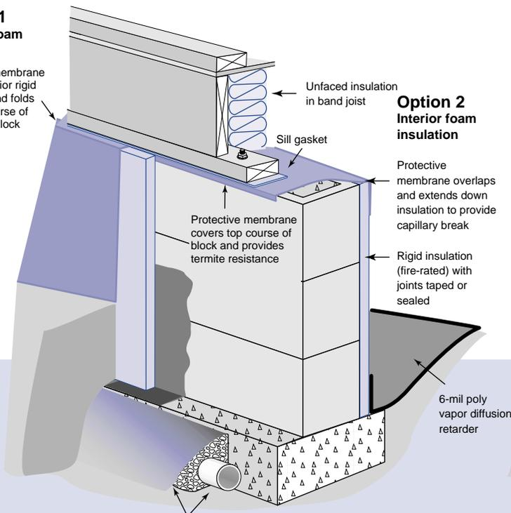
Perforated drainage pipe is embedded in gravel, covered with filter fabric, and located at lower perimeter of foundation footing to provide drainage.
