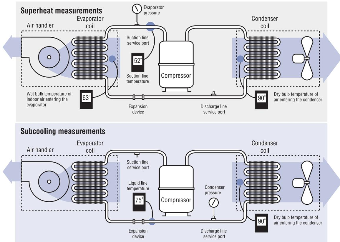
Once the system has been properly evacuated, refrigerant can be weighed into the system per specifications or a pre-charge stored in the outdoor unit can be released (package systems are most often shipped fully charged). In both cases, account for any additional charge needed for refrigerant line lengths.
