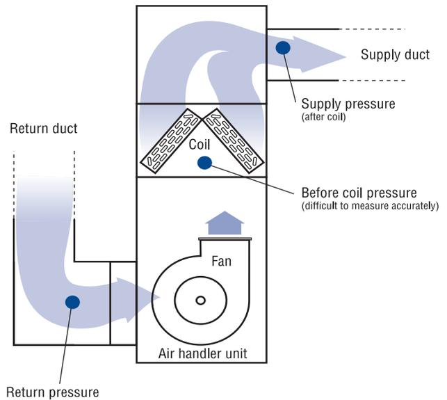
usually be based on the pressure between the return plenum and the area either before or after the indoor coil. Measuring the pressure before the coil is difficult, so it may be easier to calculate it by measuring the pressure after the coil and compensating for the pressure drop across the indoor coil.
