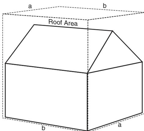
The catchment area of the roof is a simple calculation of width x length of the house. To find how much rain will be collected, take the area of the roof, multiply by the annual rainfall amount, then multiply by .5618 to arrive at the average number of gallons yearly.
